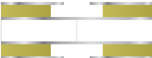
The pipe insulation is "cut back" typically 600mm. The outer carrier pipe has a 250mm (typ) gap to allow welding of inner process pipe.
