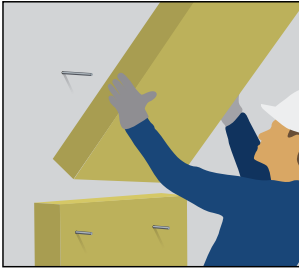
Mount Rockwool Insulation for fire protection.
