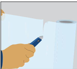
Cut foil in suitable lengths + overlap (min. 100 mm).
