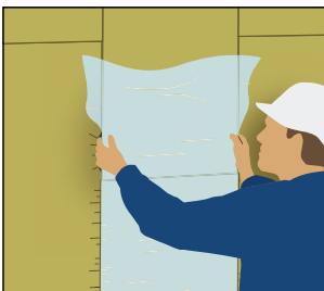
Or with an overlap of min. 10 mm attach foil to insulation by wrapping around slab.
